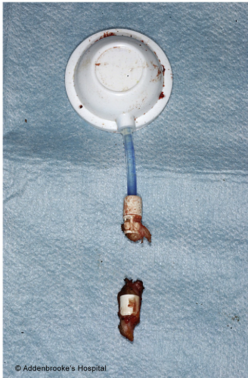
Figure 7 Intra-operative photograph of an injection port whose fill tube was found to have detached from the connector with an ingrowth of scar tissue. This had prevented expander inflation. It was attributed to a technical error, possibly clamping of the tube with a haemostat at the time of reconstruction.
